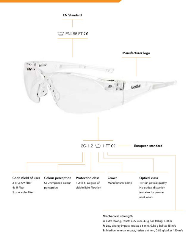
A: High energy impact, resists a 6 mm, 0.86 g ball at 190 m/s
