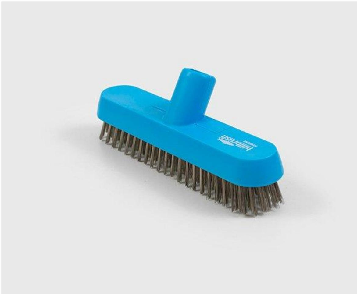
230mm floor scrub, Polypropylene block, filled rust proof 0.31mm type 316 stainless steel wire. Our most abrasive scrub. This brush is typically used for scouring concrete. A resin set version is available, B1342RES. Recommended handle ALH7. A wood backed steel filled broom is also available, see 1130/12.
