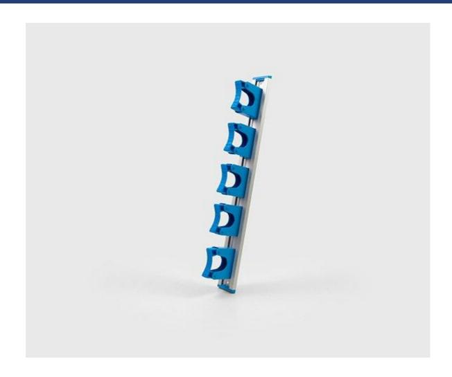
515mm Aluminium rail complete with 5 x HOLD1 holders, matching end inserts, with fixing screws and rawl plugs. The holders in this product contain rubber, which can lose its elasticity or even break if repeatedly exposed to oil. If you need a hanger for use in an oily environment, try a RAIL500 with HDHOOK1 hooks only, or our one piece hanger WLBR1, which are not affected.
